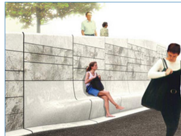
An example of a seat wall that is integrated in a retaining wall.
