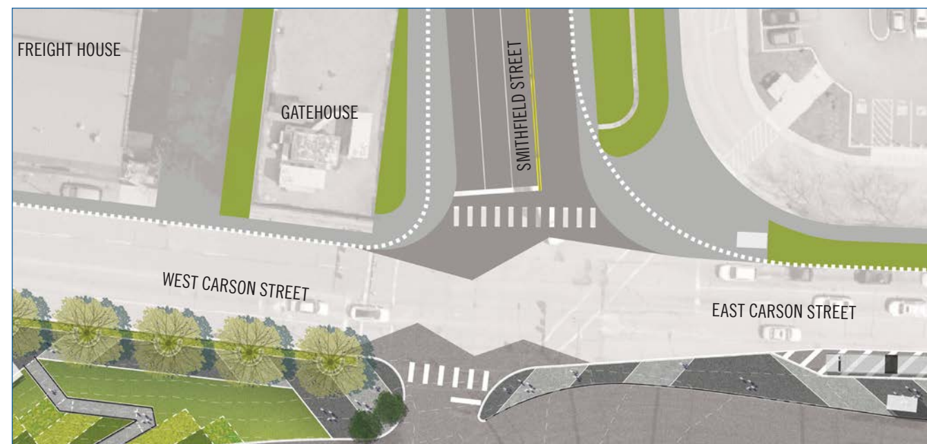
Diagram highlighting the possible reallocation of roadway space along the bridge's south side to reduce crossing distances. The dashed white lines highlight the existing location of the curb along Smithfield Street.
