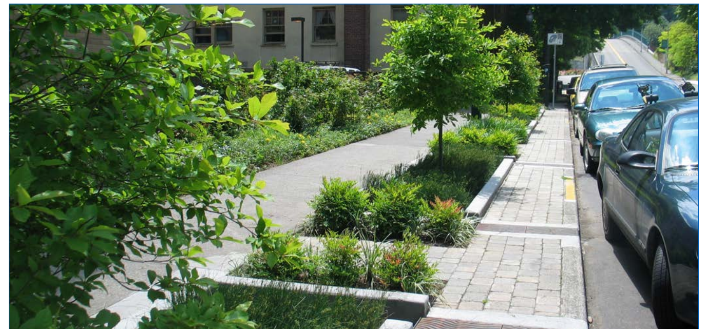
Green infrastructure improvement to streetscapes using vegetation to buffer pedestrians from traffic Source: njfuture.org
