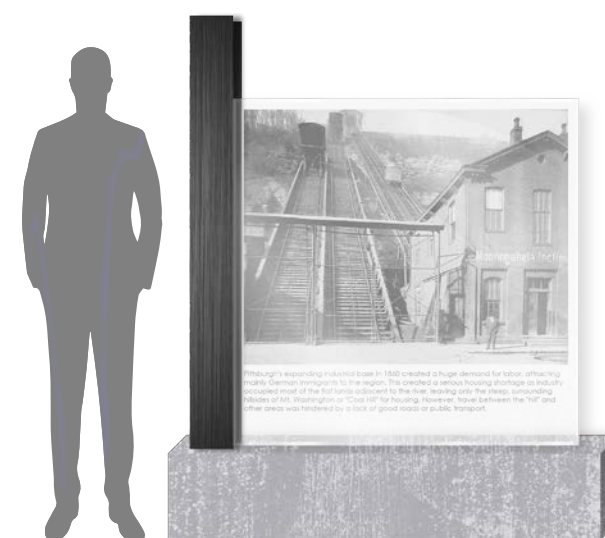
Proposed concept for displaying historical imagery at the plaza adjacent to the Monongahela Incline Lower Station - using a solid concrete base for weathering and a raw steel support beam to anchor the glass exhibit showcasing transit history
