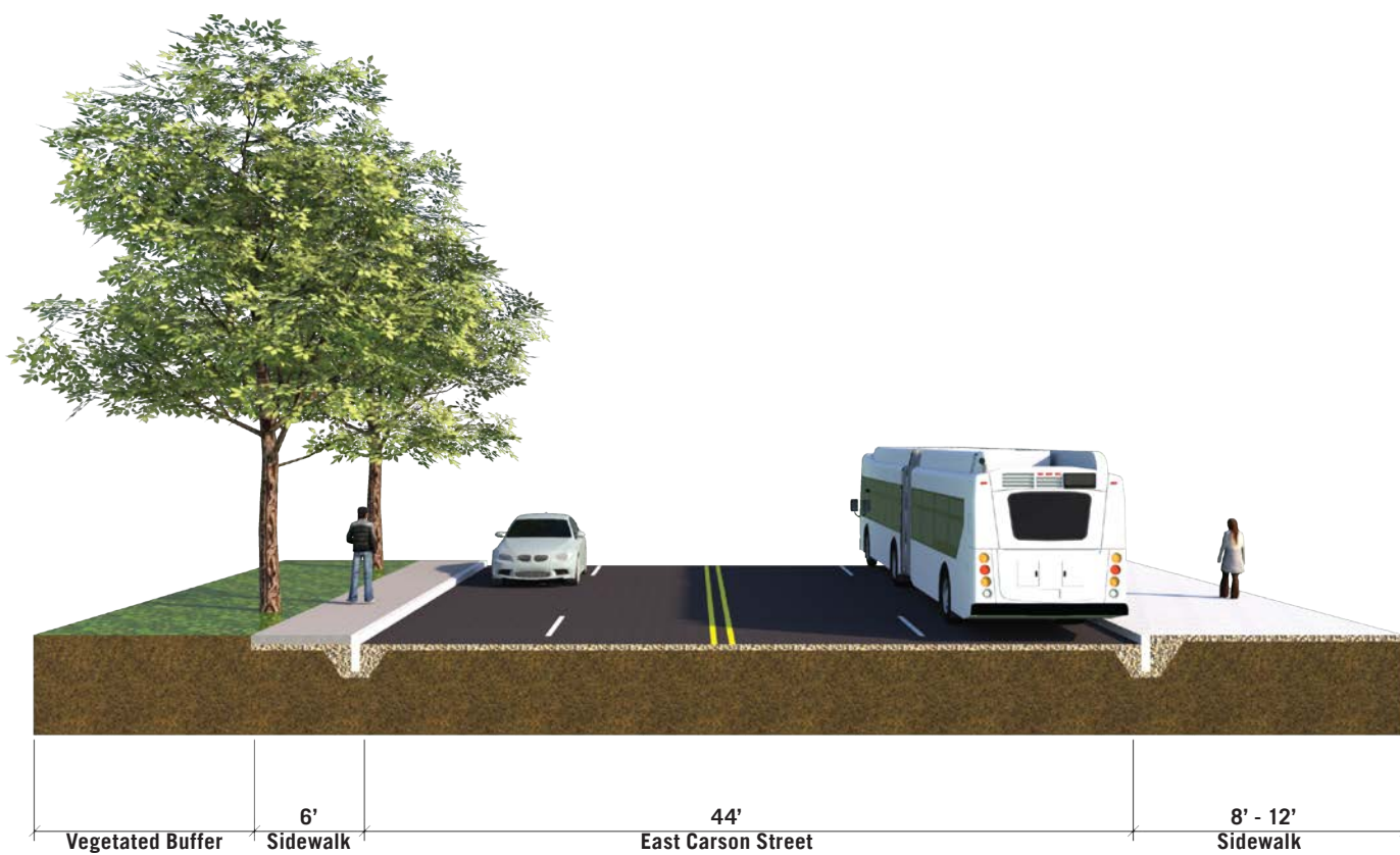
Existing Roadway Cross Section - East Carson Street
