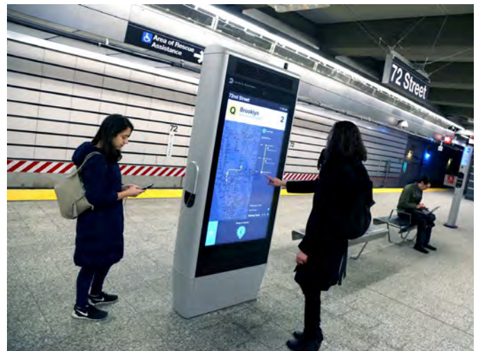
Interactive wayfinding and transit schedule kiosk with integrated device charger on platform. Product by Intersection in New York City
