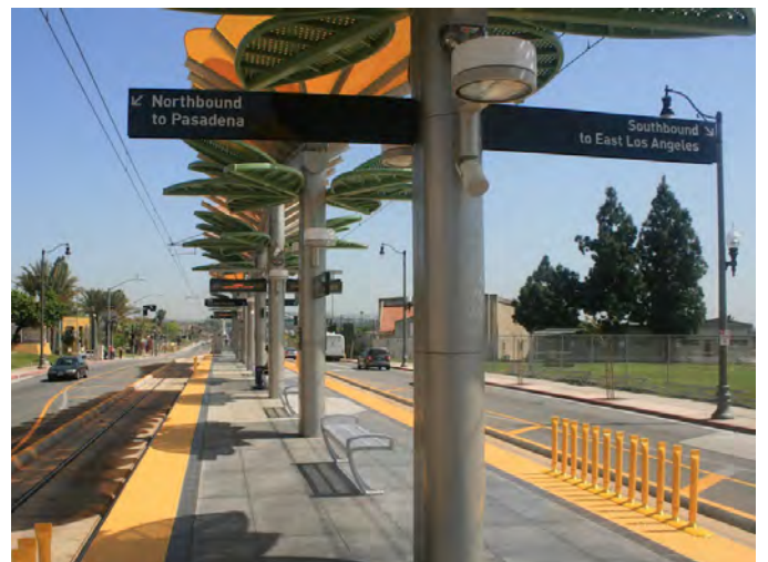
For center mounting stations, place Directional Signage on the same vertical posts perpendicular to the tracks. East LA Civic Center Station, Los Angeles
