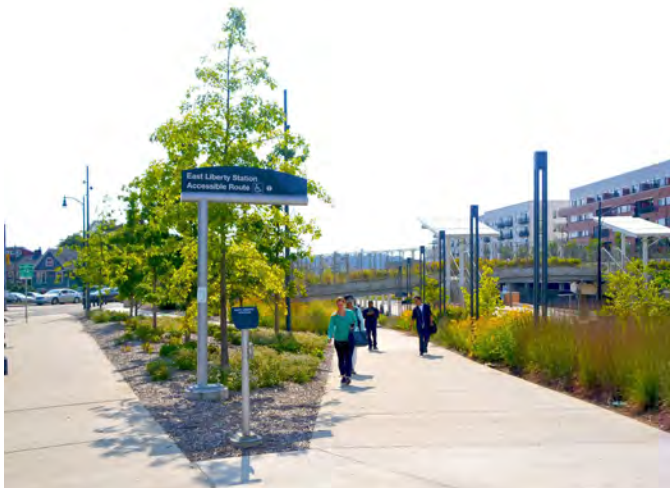
ADA Signage should be placed along the station property to direct arriving riders the accessible routes to the platform. East Liberty Station, Pittsburgh
