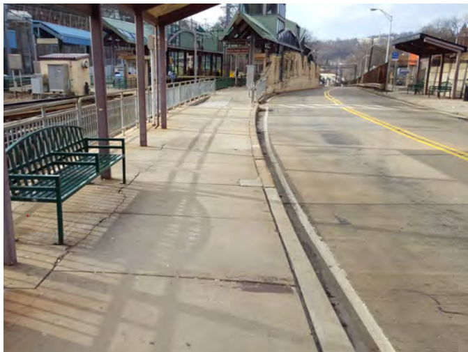
Place adjoining light rail and busway stops direct & close to each other to facilitate transfers and limit confusion. South Hills Junction Station, Pittsburgh
